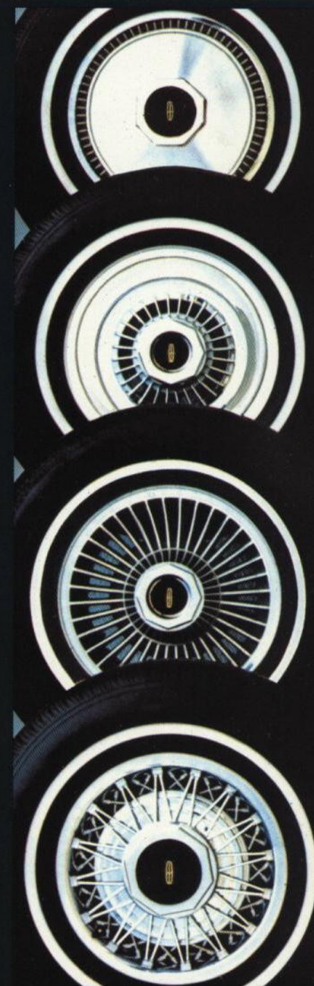
Shown, top to bottom, are standard wheel cover and these options: forged aluminum wheel, turbine-style cast aluminum wheel and wire wheel cover.
